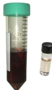
**Figure 3.** 24 mL of the loading solution in a 50 mL falcon (left), and 24 mL of loading solution concentrated using **AFFINIMIP® SPE Glyphosate** (right).
